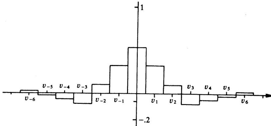
FIG. 3. Sampling weights for 3 to 1 data compression, assuming linear reconstruction.
