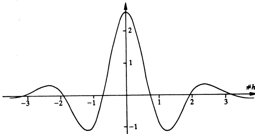
FIG. 2c. Sampling kernel for cubic spline reconstruction.
