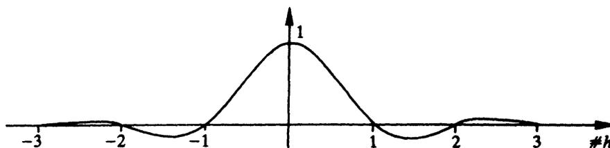
FIG. 1. Basis cubic spline.
