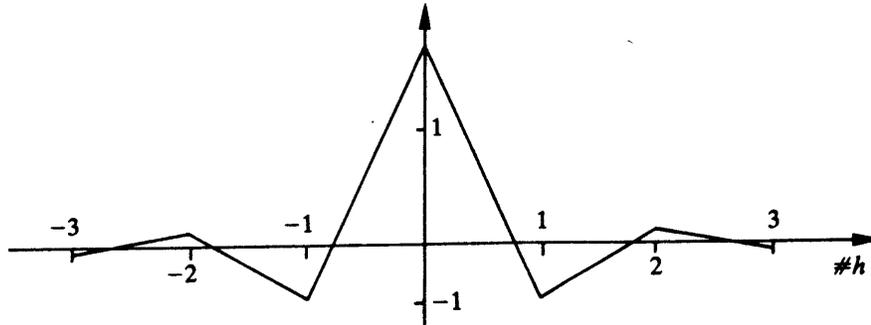
FIG. 2b. Sampling kernel for linear reconstruction.
