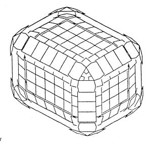
Figure 5: Display of the unit planes comprising the surface of a coarsely sampled cube.
