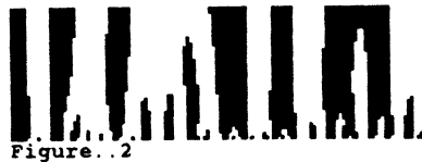
Figure 2. The sign of the scale-space filtered data shown in Figure 1. Positive regions are shown in white, negative in black, and values very near zero are in gray. The zero-crossing occur on the borders between black and white regions and within gray areas.
