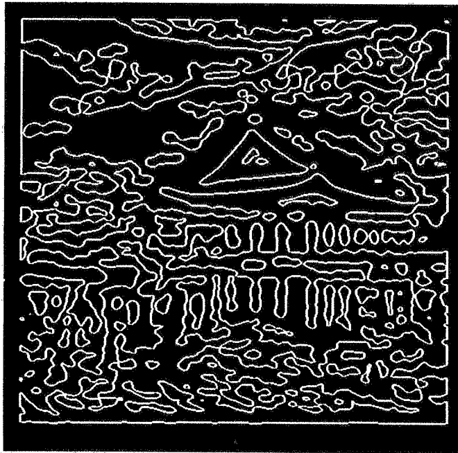
Image 3. The zero-crossings of the Laplacian-of-Gaussian filtered version of the image in Image 1, where the Gaussian has standard deviation \sigma corresponding to 4.9 pixels.
