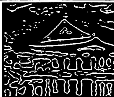
Image 5. The zero-crossings of Image 3, retaining only those zero-crossings that pass the "Berzin's test," namely those for which \nabla f \cdot \nabla(\Delta f) < 0 .
